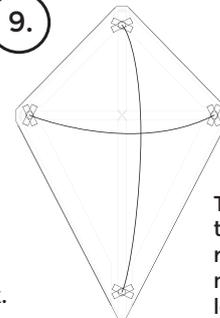
Thread the string through holes and reinforce with masking tape, leave some slack in the string, as this is the sting that will be attached to the kites main line.
